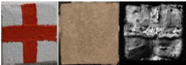
Figure 3. Sequence of images from unobscured to obscured, and then imaged with THz system
