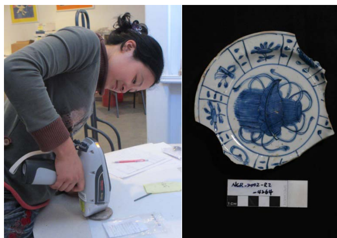
Figure 2. Analysis with pXRF of a blue-and-white porcelain fragment.
