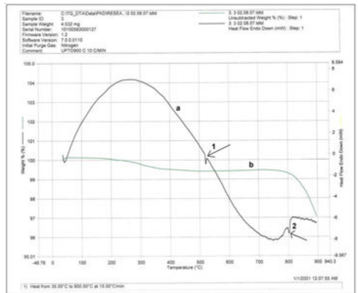
Figure 10. (a) Data for DTA indicating small endo peaks at 520 °C and 802 °C marked by arrows, (b) Data for TGA do not provide substantial information.
