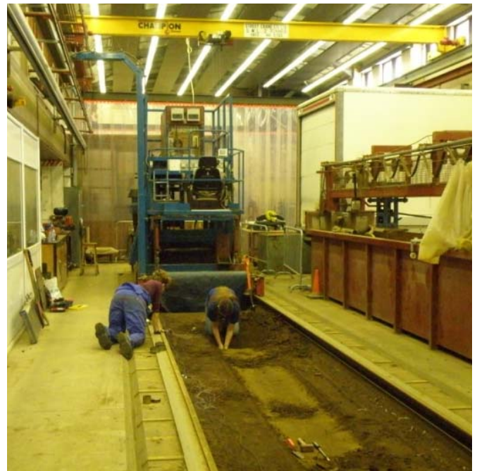
Figure 1. Soil bin at Cranfield University, showing the tyre rig set to exert a specific pressure and the re-excavation of artefacts after one pass of the rig.
