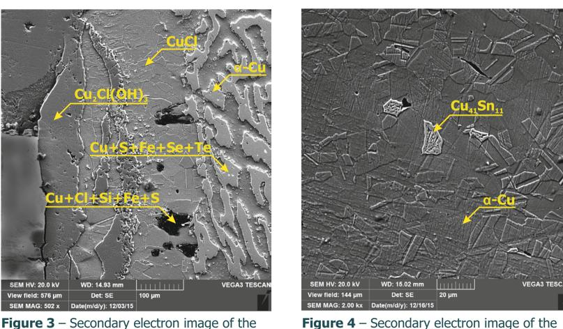
microstructure of sample 2169 microstructure of sample 2167
