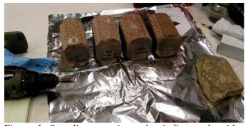
Figure 1. Sampling experimental grinding tools with a portable drill fitted with diamond-embedded, solvent cleaned, core bit
